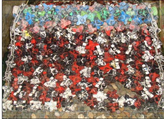
In test AII\_2 the Xbases displaced a significant distance resulting in excessive settlements in the armour layer of the leeward slope. The test is executed again (test AII\_2\_1) with fixed Xbases in lateral direction (see Figure 5.7).
