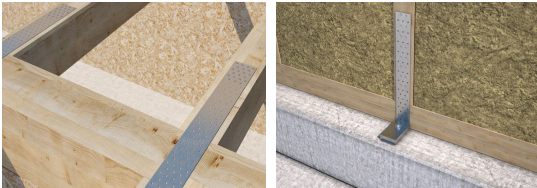
Figure 2.6: Joint with steel nails [55]
