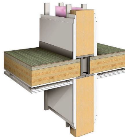
Figure 5.5: Type X gypsum layers around a column [45]
