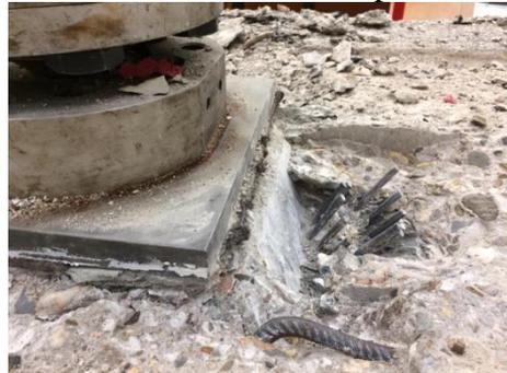
Failure, top view showing anchorage of prestressing tendon
