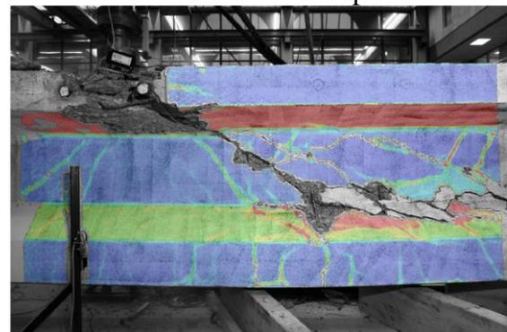
Failure by local crushing of concrete in the top flange
