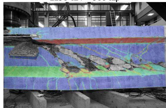
Failure by crushing of concrete in compression field in the web
