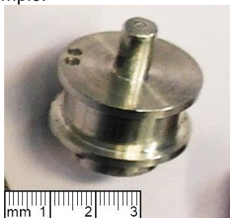
Figure 70: Pulley with Cable Loop Holes
