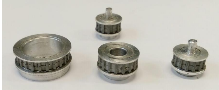
Figure 74: Completed Timing Pulley
