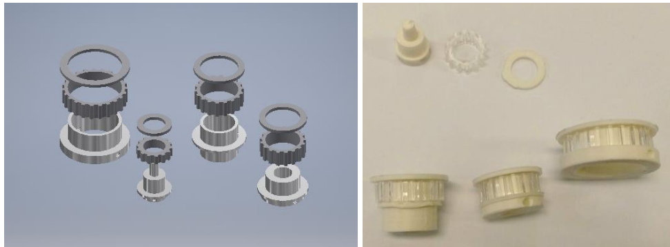
Figure 73: Timing Pulley Prototype Design
