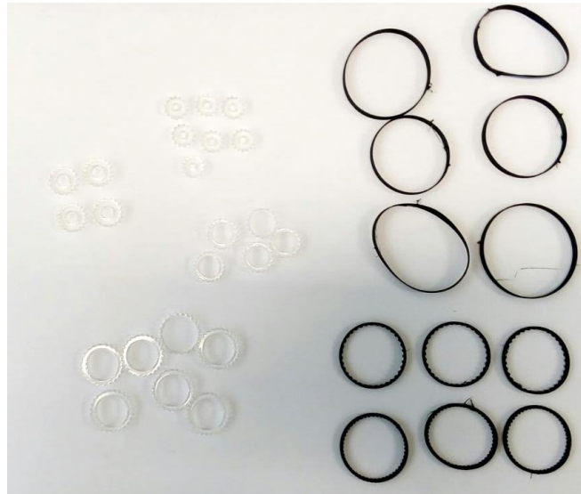
Figure 64: Timing Pulleys and Belts Prototyped
