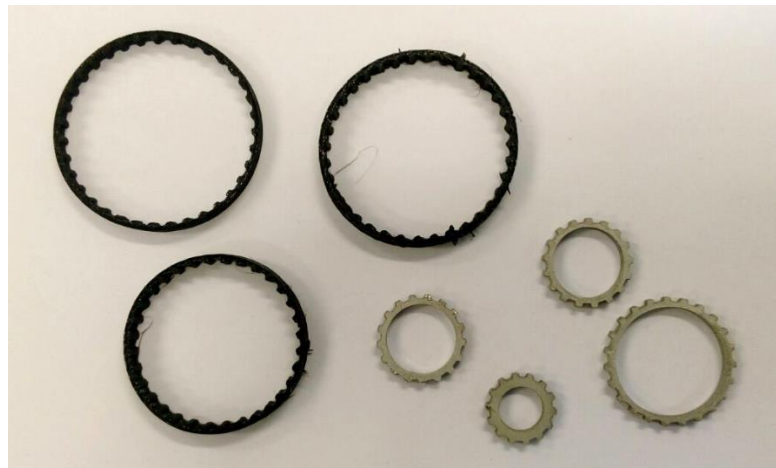
Figure 65: Timing Belt and Pulleys Selected
