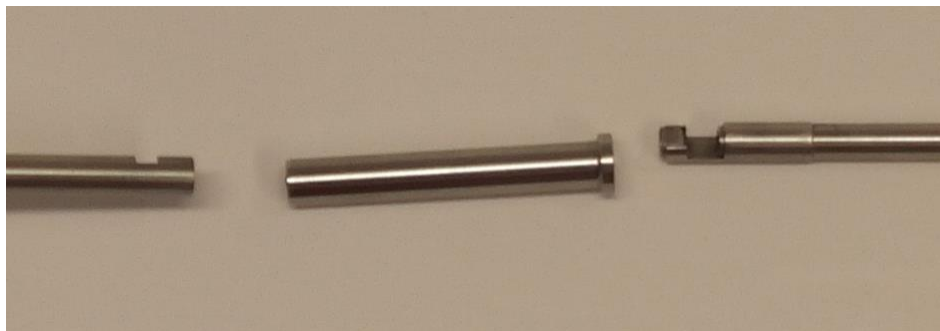
Figure 10: Instrument Attachment/Removal Coupling
