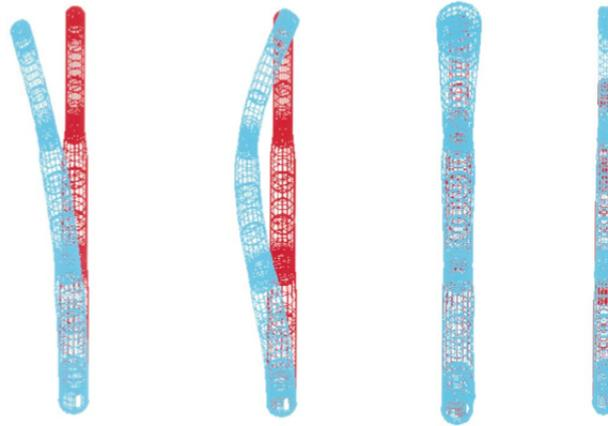
Figure 3.4: The first four eigenmodes of an offshore wind turbine tower. These eigenmodes are from left to right: first bending mode, second bending mode, torsion and axial displacement [11].
