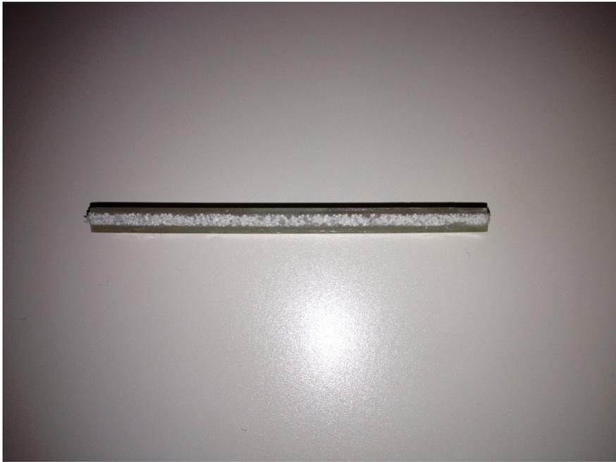
Figure B.5: The final appearance of the sandwich structured composite samples.
