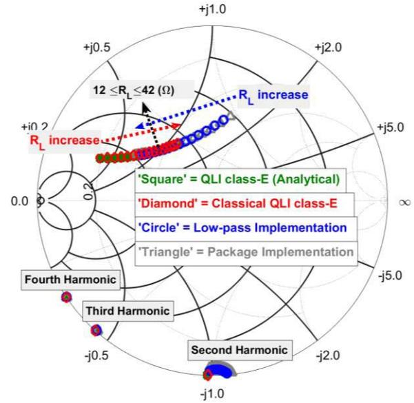
Fig. 3. Admittances plot (fundamental, second, third, and fourth harmonics) as a function of  $R_L$  swept from  $12 \leq R_L \leq 42$  ( $\Omega$ ) for the QLI class-E: analytical solution using (9), simulation response of the circuits given in Fig. 1(a) and the low-pass implementation is given in Fig. 2(a) and package implementation estimation is given in Fig. 2(b).
