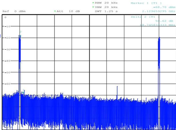
Fig. 16. Measured amplifier full output spectra directly captured from spectrum analyzer (SPA) when driven with 5-MHz LTE signal at 2.12- and 2.52-GHz (BW = 400 MHz) SPA SPAN = 500 MHz.
