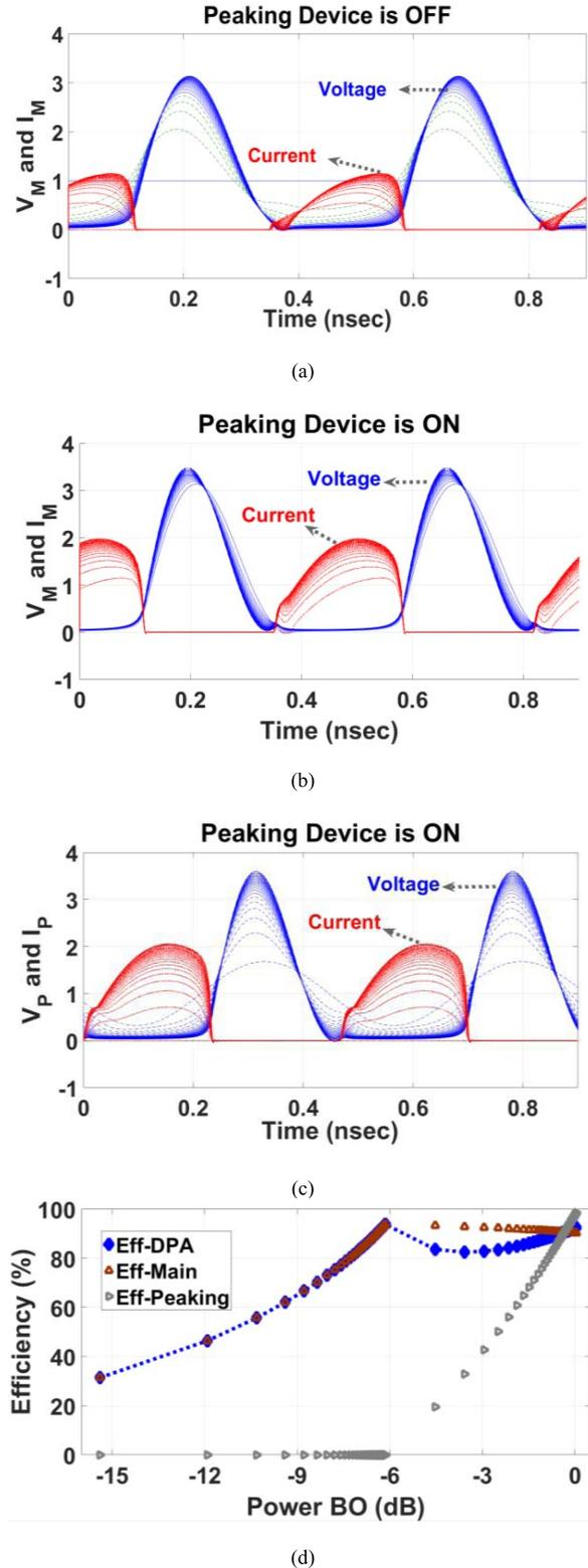
Fig. 7. Simulated intrinsic voltage and current waveform at drain terminal of Main and Peak devices (QLI class-E) in Doherty configuration. (a)  $V_M$  and  $I_M$  at BO power levels (peak is OFF). (b)  $V_M$  and  $I_M$  at maximum power levels (peak is ON). (c)  $V_P$  and  $I_P$  at maximum power level. (d) Efficiency as a function of BO power level.
