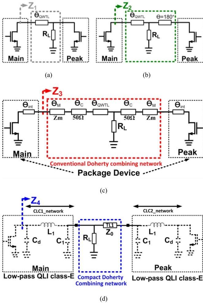
Fig. 6. (a) Classical class-B Doherty. (b) Modified wideband class-B Doherty. (c) Conventional class-B Doherty configuration using package device with  $\Theta_{int}$  internal rotation. (d) Proposed compact Doherty configuration featuring QLI class-E operation.
