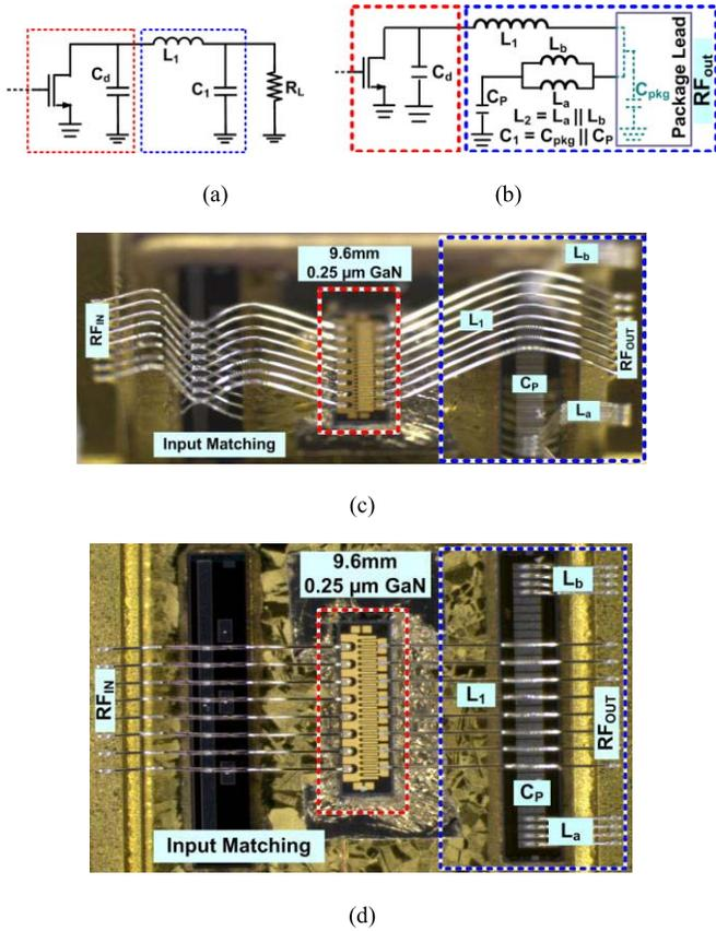
Fig. 2. QLI class-E low-pass circuit configuration. (a) Simplified schematic. (b) Schematic for package implementation ( $L_a$  and  $L_b$  are very small). (c) Side view and (d) top view of physical network implemented inside standard Ampleon SOT1135A package.
