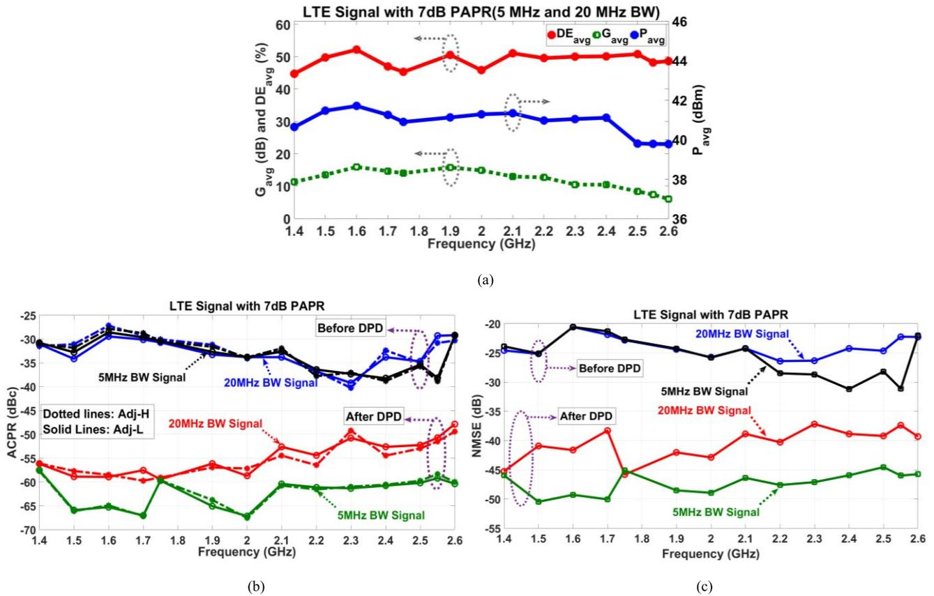
Fig. 13. Dynamic measurement of dual input DPA with LTE 5- and 20-MHz modulated signals with 7-dB PAPR. (a) Average output power ( $P_{avg}$ ), drain efficiency ( $DE_{avg}$ ), and gain ( $G_{avg}$ ) versus frequency. (b) ACPR before and after DPD versus frequency. (c) NMSE before and after DPD versus frequency.
