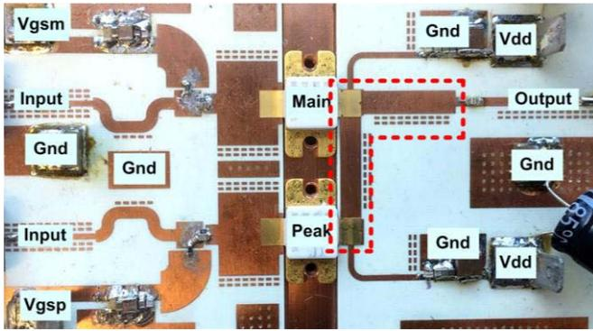
Fig. 10. Hardware prototype of the proposed compact wideband DPA featuring QLI class-E operation.
