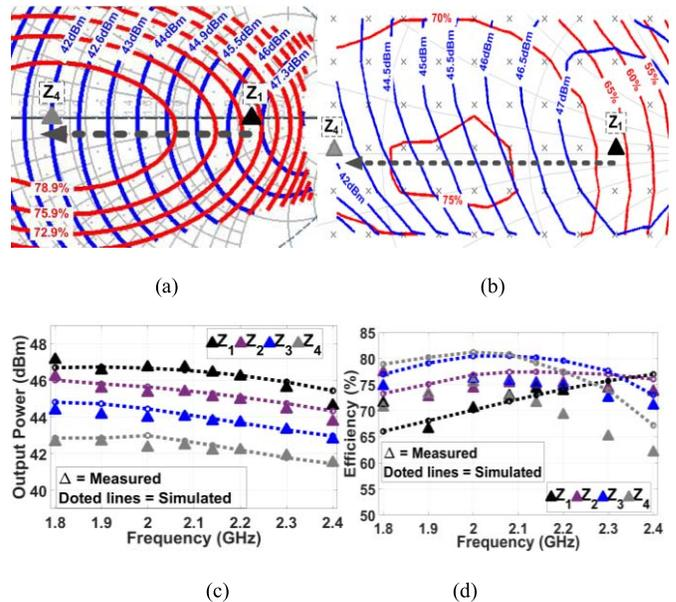
Fig. 5. 9.6-mm 0.25- $\mu\text{m}$  GaN QLI class-E device results. (a) Simulated LP data at 2.14 GHz with  $Z_{\text{ref}} = 10 \Omega$ . (b) Measured LP at 2.14 GHz with  $Z_{\text{ref}} = 10 \Omega$ . (c) Comparison between simulated and measured output power versus frequency at different impedance levels. (d) Comparison between simulated and measured efficiency versus frequency at different impedance levels.
