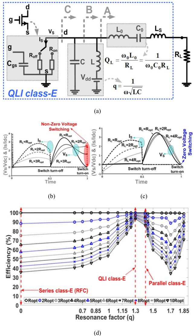
Fig. 1. QLI class-E. (a) Principle schematic of the finite dc feeds inductor configuration with series resonator. (b) Waveforms when the resonance factor  $q = 0$  and (c) when  $q = 1.3$ . (d) Efficiency as a function of resonance factor  $q$  at frequency = 2.14 GHz for loading conditions that represent a multiple of the optimum load value for reaching MXE.
