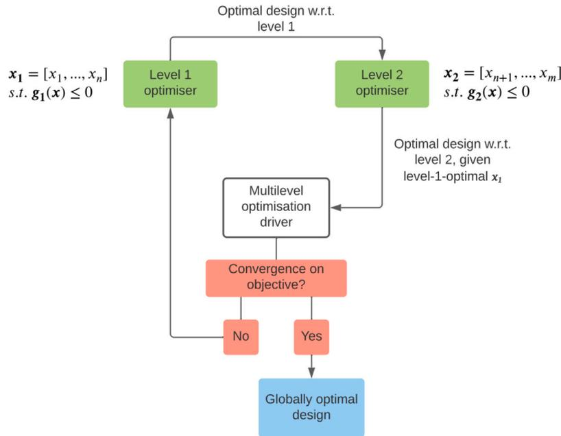
Fig. 13. Multilevel optimisation approach with decomposition of the design space into two disjoint sets  $x_1$  and  $x_2$ . Source: Reproduced from Ashuri et al. (2014).
