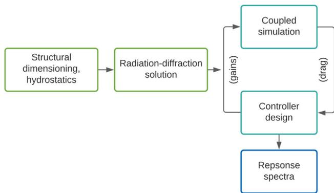
Fig. 10. FOWT system-level design optimisation scheme including drag-control loop. Source: Reproduced from Lemmer et al. (2020).
