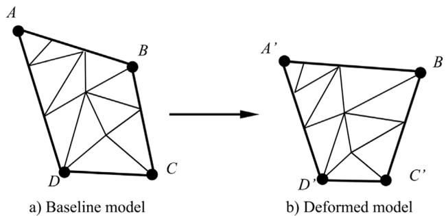
Fig. 11. Domain element method — macro element shape transformation.
