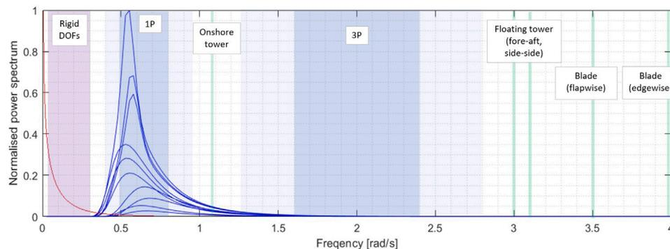
Fig. 8. Example frequency map for the IEA Wind 15MW reference rotor adapted from Allen et al. (2020). Red curve — Kaimal wind spectrum, blue curves — JONSWAP wave spectrum for a range of sea states. Dark shading for the main range, light shading for the safety margins of  $\pm 2$  standard deviations. (For interpretation of the references to colour in this figure legend, the reader is referred to the web version of this article.)
