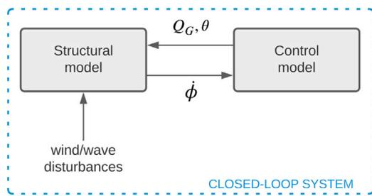
Fig. 5. Assembly of the structural and control models in one closed-loop state-space system through input/output pairs: generator torque  $Q_G$ , blade pitch  $\theta$  and rotor speed  $\dot{\phi}$ .
