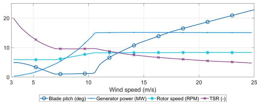
Fig. 7. IEA 15MW controller regulation trajectory — variable speed variable pitch strategy. Source: Adapted from Evan et al. (2020).
