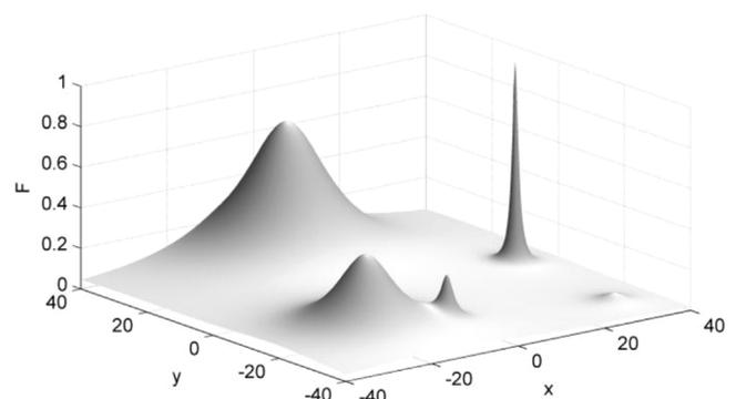
Fig. 9. Cumulative Multi-Niching Genetic Algorithm (CMN GA) 2D design space exploration — multiple local maxima can be seen.
