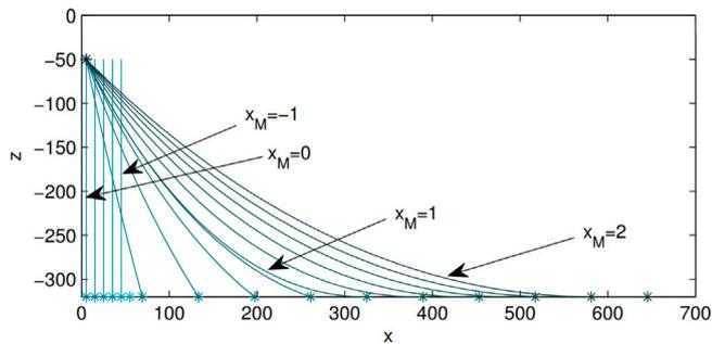
**Fig. 6.** Example of mooring line profiles for the line shape parameters  $x_M \in [-1, 2]$ . Source: Reproduced from Hall et al. (2013).
