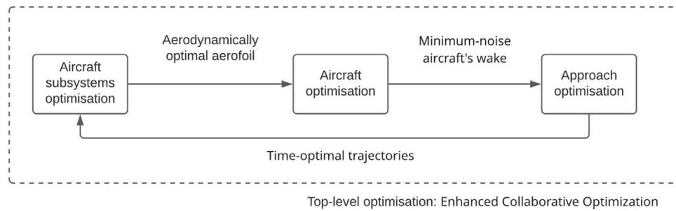
Fig. 3. Example of optimisation decomposition in aeroplane design, based on Subramanian and DeLaurentis (2016).
