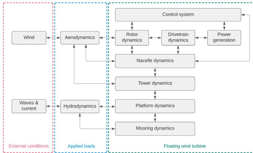
Fig. 12. Modules interface in a fully coupled aero-hydro-servo-elastic model within OpenFAST. Source: Reproduced from Jonkman (2007).
