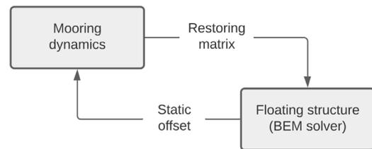
Fig. 4. Iterative approach to steady state offset and mooring restoring matrix. Source: Adapted from Tracy (2007)
