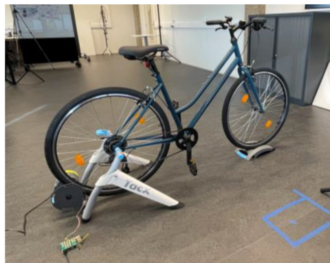
Figure 3: The virtual reality cycling simulator.
