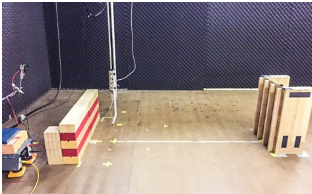
FIG. 10 Measurement set-up in a 1:50 down scaling at the measurement facilities at TU Delft, picture by the author.
