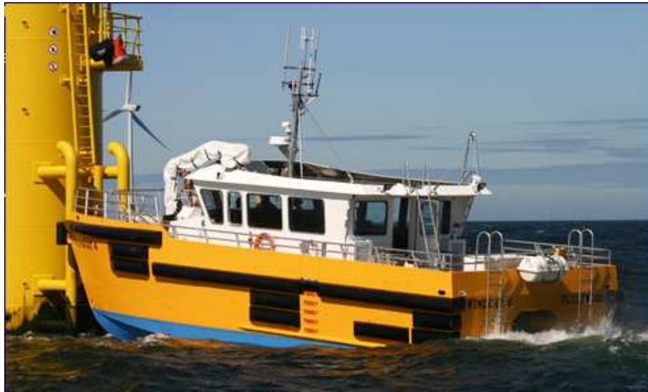
Figure 39. Simple access system (WindCat)
