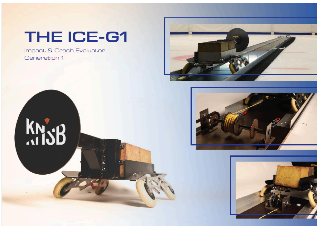
Figure 1.7: The Impact & Crash Evaluator 1st Generation (ICE-G1), a circular ram designed to be launched at padding on ice rinks (Beets et al., 2024)
