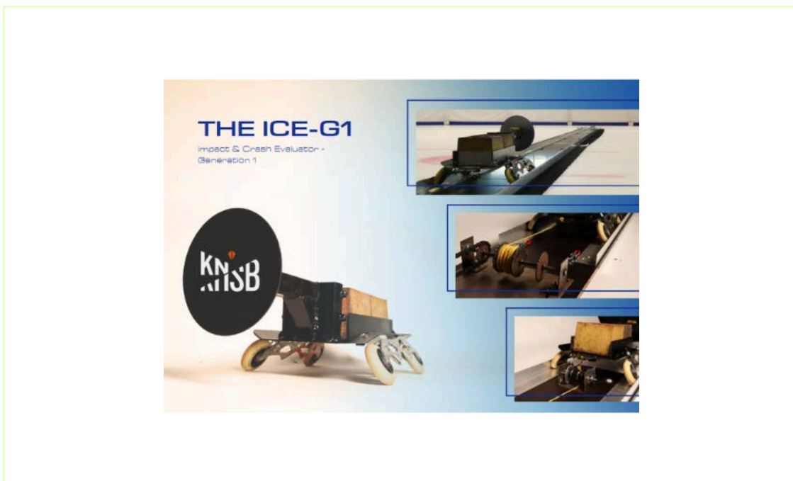
image / figure 2 The sled with a rigid ram of the ICE-G1
