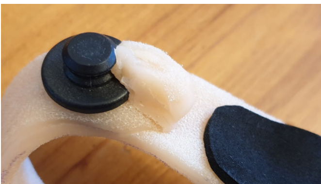
Figure 51: Solution to the axial asymmetrical male part.
