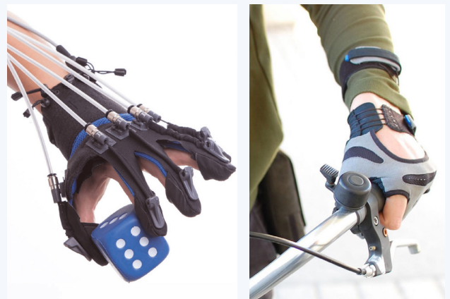
Figure 27: Left, Gloreha sinfonia (Gloreha, n.d.) a robotic device for hand rehabilitation. Right, Carbonhand by Bioservo (Cypromed, 2020).
