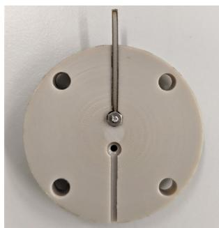
(b) The cathode front endplate fitted with the connection rod at the top side.
