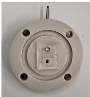
(a) The cathode front endplate including the electrode holder connected at the top connection.
