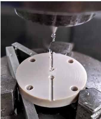
(a) Making the connection rod slots on the milling machine.
