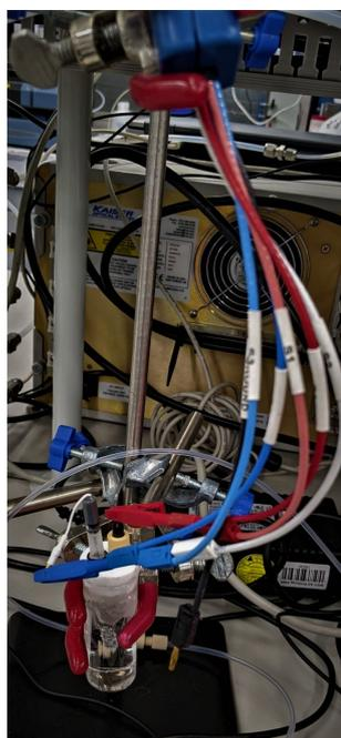
Figure B.19: An illustration of the connections and set-up of the OCP testing of the reference electrode (right) against the master reference electrode (left).
