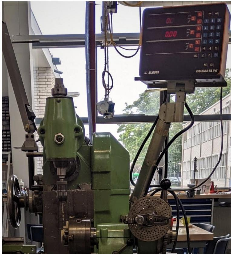
Figure B.16: A visual representation of the digital readout machine on the milling machine.
