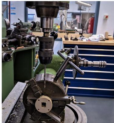
(b) Drilling the holes in the reaction chamber with the milling machine.
