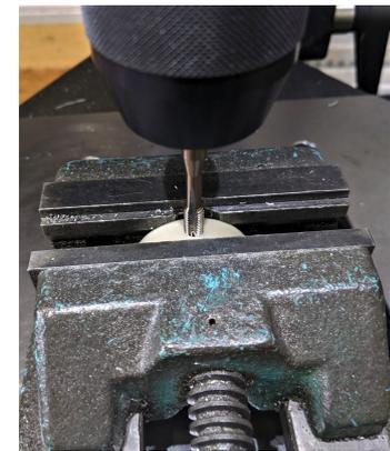
(c) Tapping the thread into the holes, with the drilling machine
