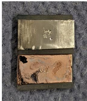
(b) The Cu and Ag electrodes after the PEIS measurements.
