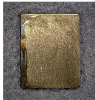
(c) The nickel electrode after conversion testing with the Ag electrode electrically connected as cathode.
