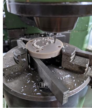
(b) Making the o-ring grooves on the milling machine.
