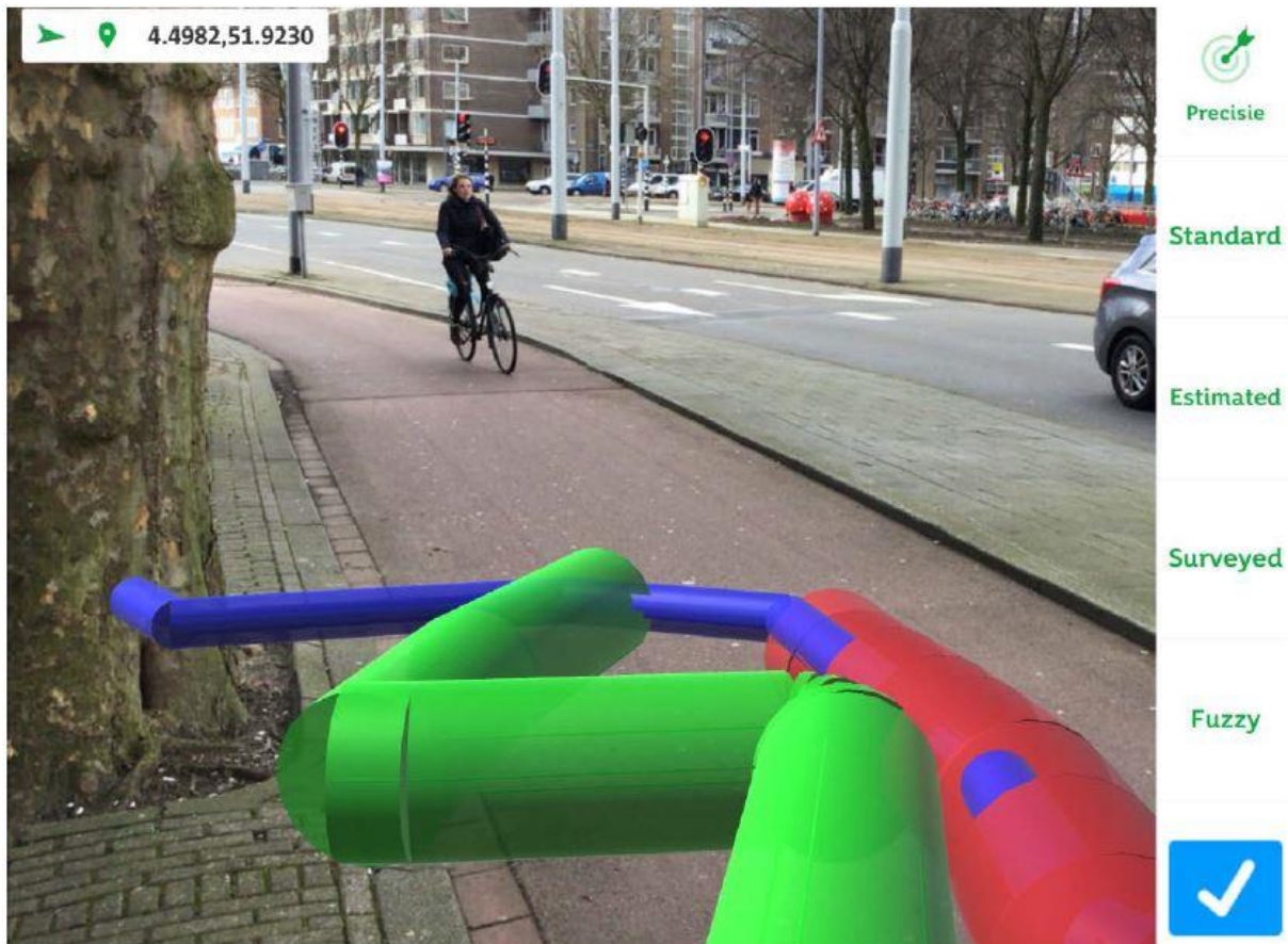
Figure 26 Augmented reality and fuzzy concepts to enable the 3D-representation and visualization of uncertainties for underground utility data (olde Scholtenhuis et al. 2017)
