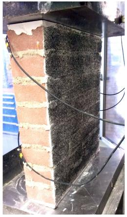
Figure 19. Wallet for a compression test in the testing rig. The front face of the wallet appears painted for monitoring with photogrammetry.
