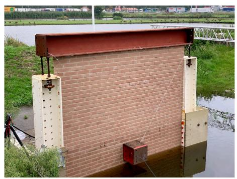
Figure 10. Object swinging against the wall to simulate 'hard' debris.
