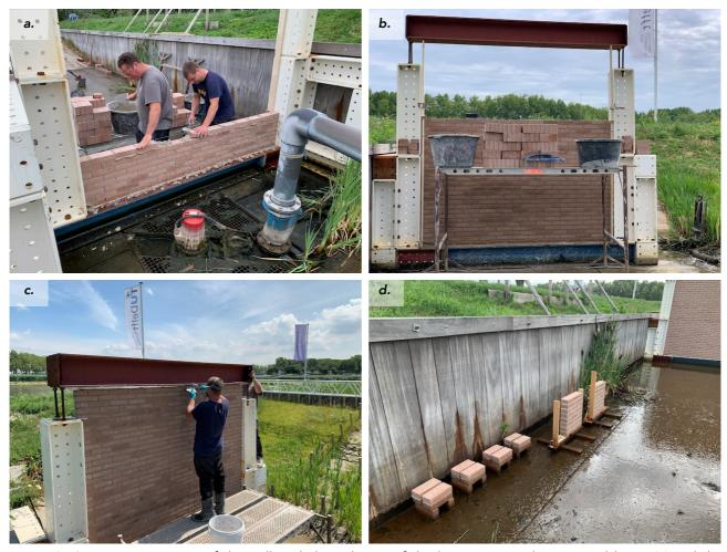
Figure 8. Construction process of the wall, including glueing of the last course to the top steel beam (c) and the companion specimens (d).
