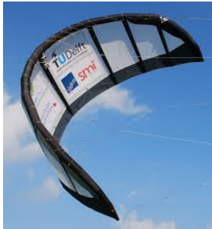
Figure 2.2: One of the LEI kites designed and used by the TU Delft AWE group for power-generation
