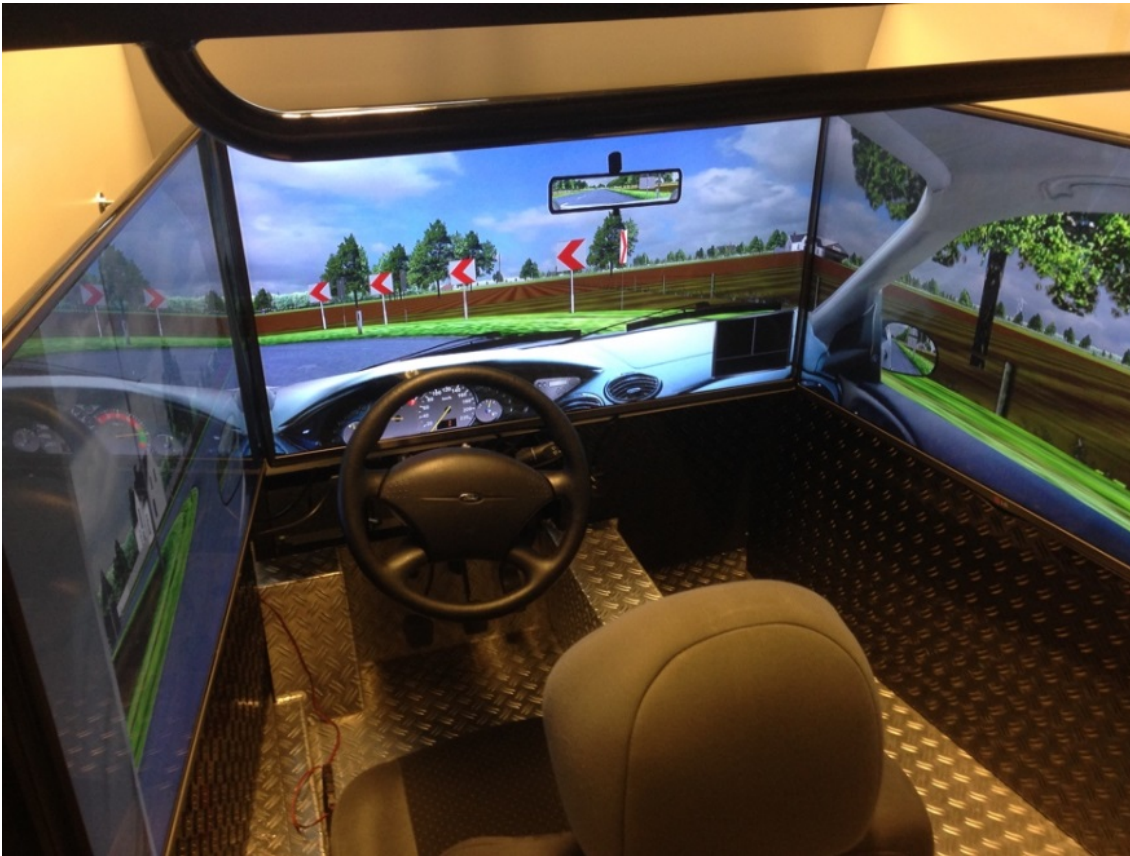
Figure 1. The driving simulator used in this research. In all trials, the screens were turned off and participants wore headphones.
