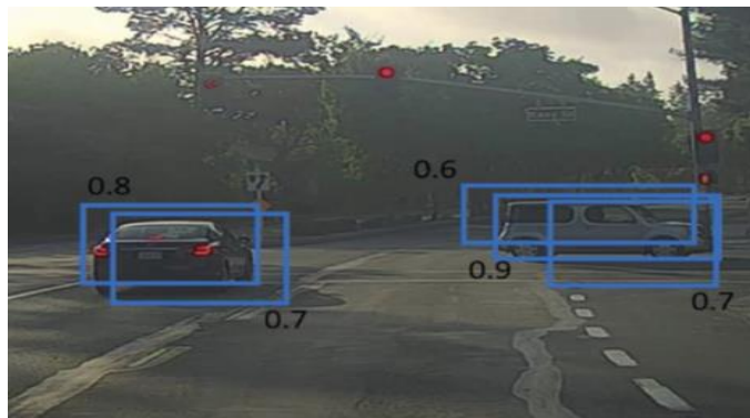
Figure D.2.3 Example of multiple detection with different probabilities for the predicted bounding boxes (image taken from [77])
