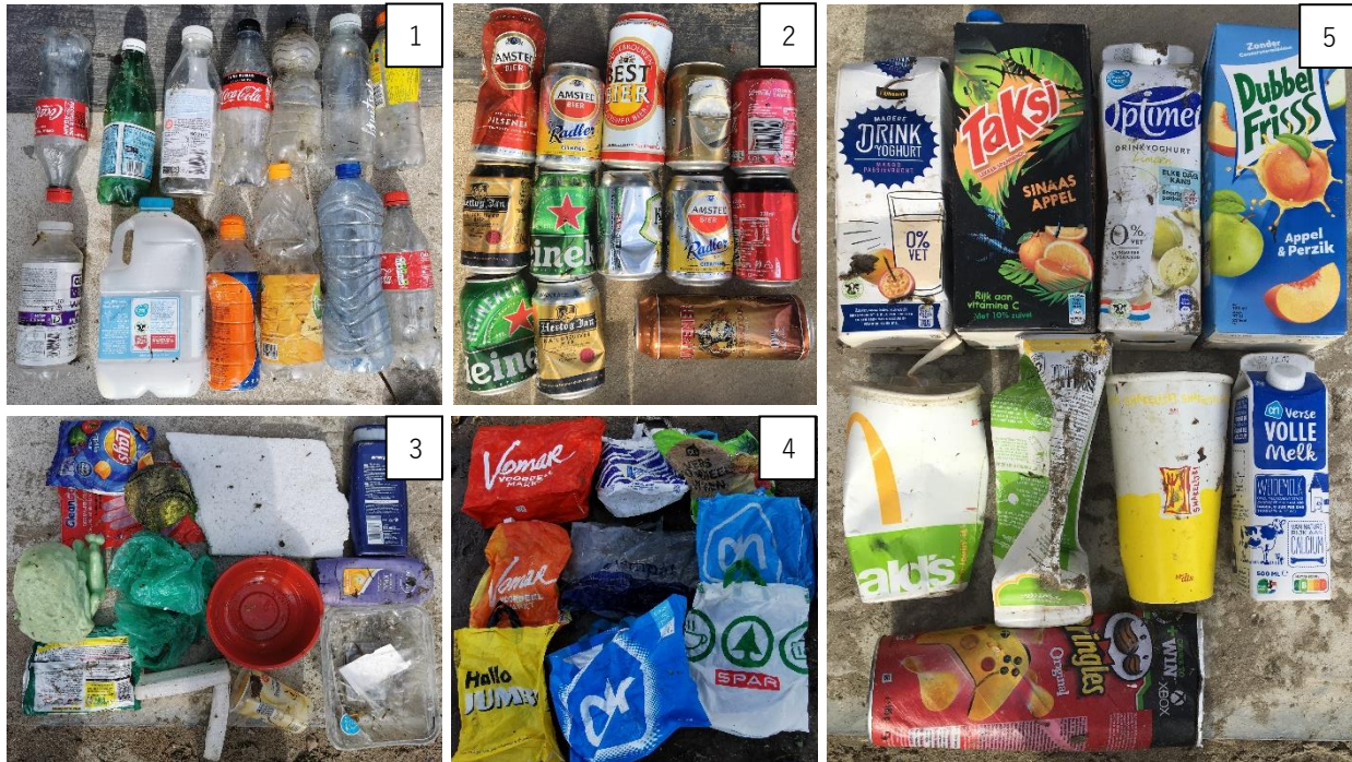
Figure 10 Impression of plastic debris objects used for the experiments at Green Village(1: Plastic bottles, 2: Metal tins, 3: Various plastic objects, 4: Plastic bags, 5: Paper)
