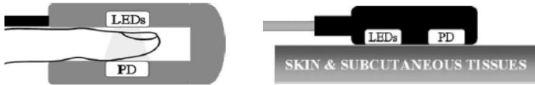
Figure 6-5: Transmittance (left) versus reflectance (right) pulse oximetry. Picture adapted from [136].
