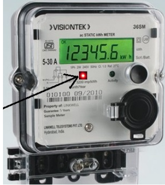
Figure 1.1: Digital meter where the arrow indicates the blinking LED.
