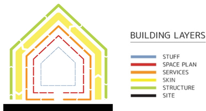
Figure 4: The building layers by Brand
