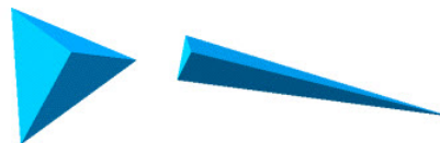
Figure 4.17: Left) Aspect ratio of unity. Right) High aspect ratio
