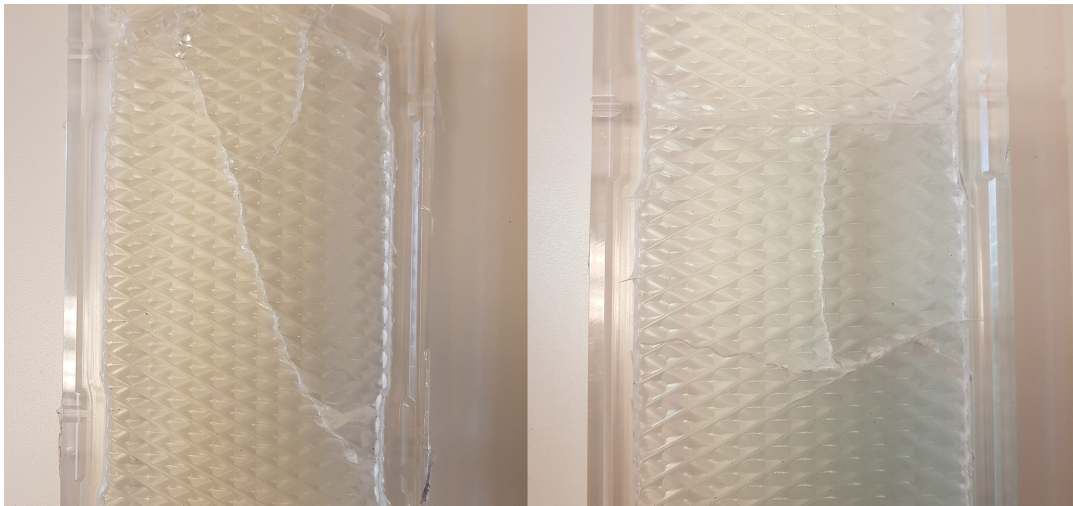
Figure 4.3: The emergence of cracks on the PMMA plate after a week
