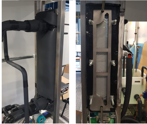
Figure 5.12: Applied insulation material to the GPHE, rear and frontal view
