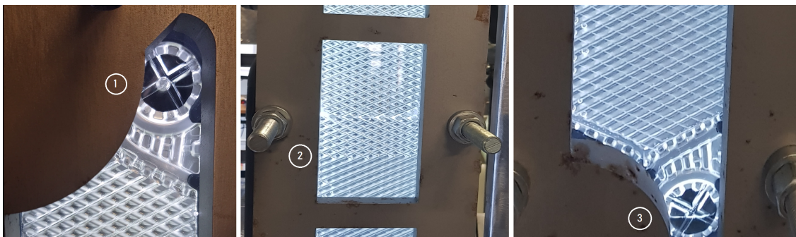
Figure 4.1: The liquid columns on the top (1), middle (2) and bottom of the plate (3)
