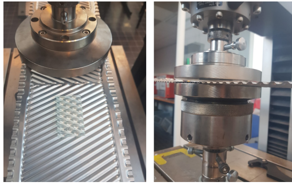
Figure 4.13: Left) Corrugated sample placed on the stainless steel plate. Right) Workbench ready to press the sample onto the steel plate
