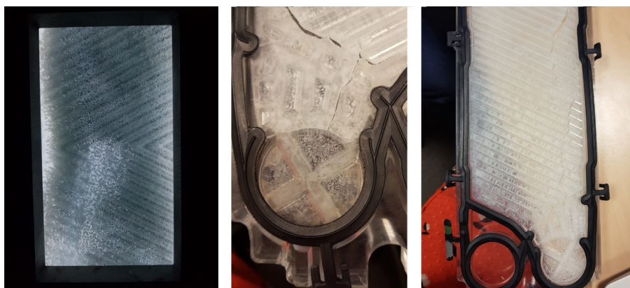
Figure 4.25: Left) The degraded material after 12 days. Middle) Degraded material of inlet zone after dismantling the plate. Right) Degraded material of corrugated zone after dismantling the plate
