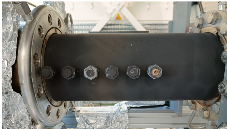
Figure 3.3: Photo of the steel chamber inserted in the combustor setup
