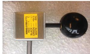
Figure 4.2: Plastic spherical knob attachment tightened to the load cell.
