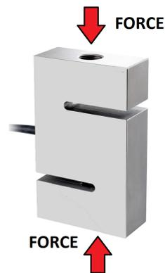
Figure 2.9: S-type load cell. If the strain gauges are glued at appropriate locations, this structure is suitable for exerting the force at the middle [30].
