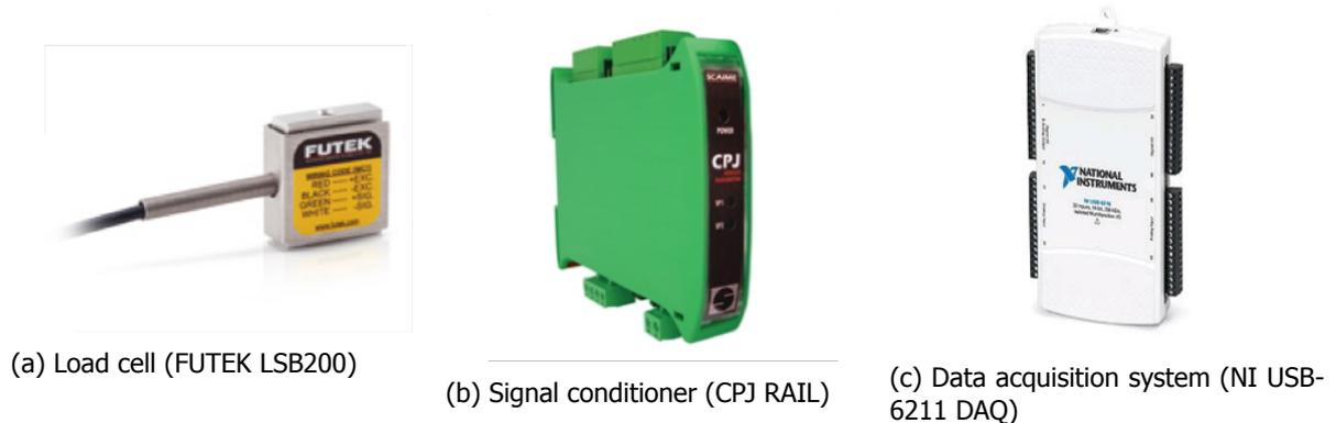
Figure 3.7: Components of the measuring system. The output signal from the load cell is amplified in the signal conditioner and converted into digital form through the DAQ device before being processed and stored in a PC using LABVIEW.
