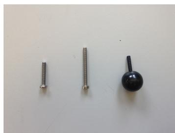
Figure 3.8: The three different sensor attachments used in this experiment: a short bolt, a long bolt and a plastic spherical knob.
