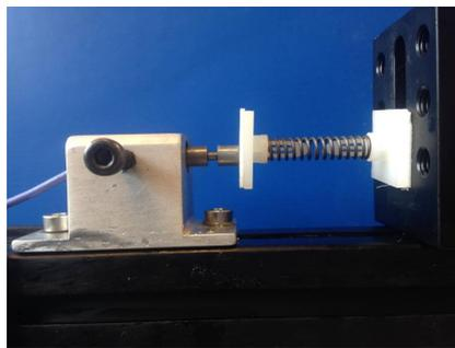
Figure 6.1: Output side of the experiment. A spring is held by a spring mounting between the piston and the rigid wall. The spring is used to simulate the target compliance.
