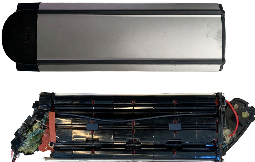
Figure 4: the inside of a Gazelle Gold battery, cylindrical cells in a robust plastic casing, control components visible on the left.
