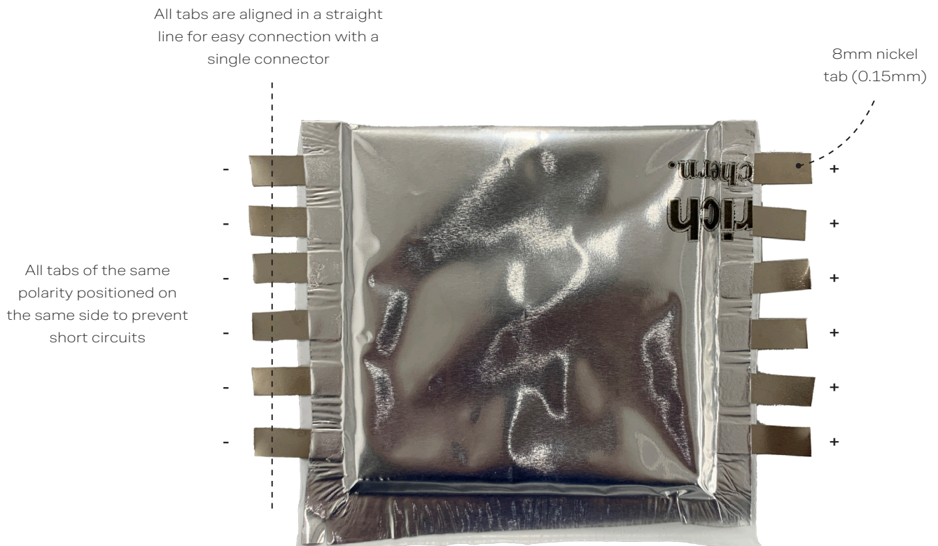
Figure 29: a prototype pouch cell highlighting the tab positioning
