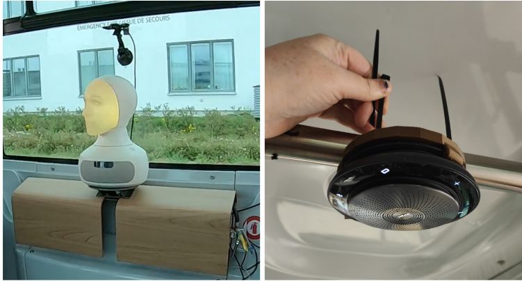
Fig. 4. Left : The Furhat agent during the experiment (marked as Robot in Figure 6). Right : A close-up of the conference microphone (marked as Microphone and speaker in Figure 6) in the ceiling of the bus that played the audio of the disembodied agent.
