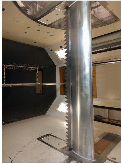
Figure 3: NACA64 3 418 model tested in the wind tunnel.
