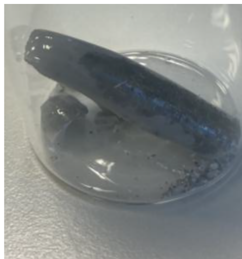
Fig. 14. A vitrified sample of surrogate materials as LiCl-ZrCl 4 in borosilicate glass.
