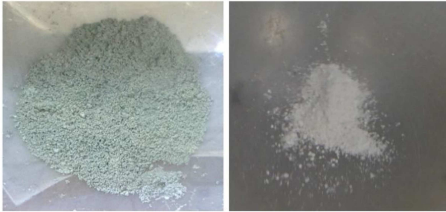
Fig. 1. Synthesized \text{PuCl}_3 and \text{ThCl}_4 salts in the lab scale quantities. Characteristic green colour of \text{PuCl}_3 on the left, and on the right \text{ThCl}_4 with characteristic white colour.
