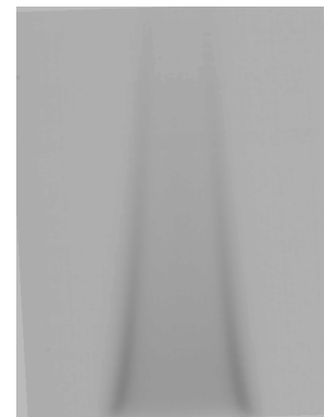
(b) Inverted chemiluminescence image from CCD camera equipped with UV filter. Exposure time t = 80\text{ms} .
