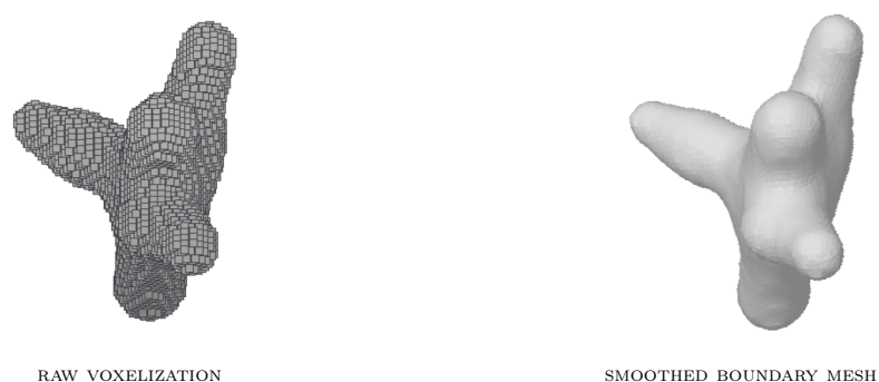
Figure 17. Implicit image-stack workflow from voxels to geometry. The left panel shows the raw binary voxelization of the 56 \times 56 \times 56 implicit field; the right panel shows the extracted and smoothed boundary triangle mesh with 11,664 faces.
