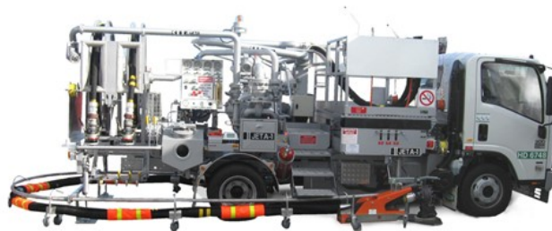
Figure A.9: An example of a hydrant dispenser truck [62].
