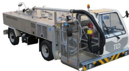
Figure A.6: An example of a lavatory service truck [81].
