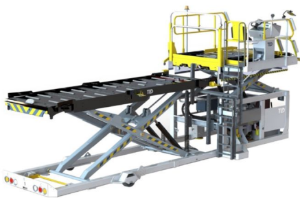
(a) An example of a lower deck loader [81].
