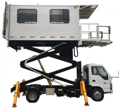
Figure A.13: An example of disabled passenger lift truck [55].
