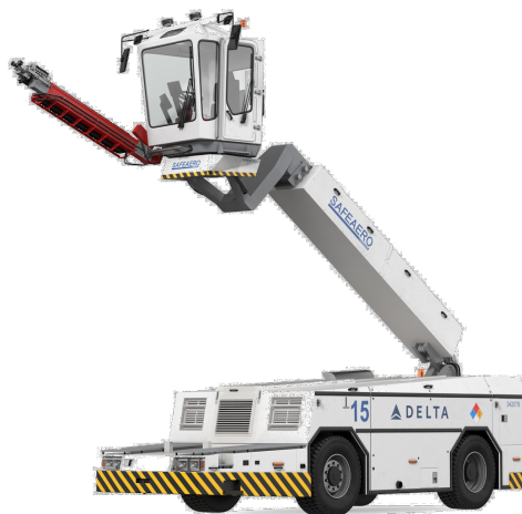
Figure A.11: An example of a deicer vehicle [82].
