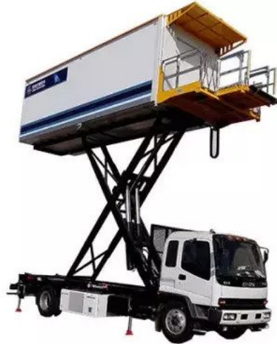
Figure A.5: An example of a catering truck [35].
