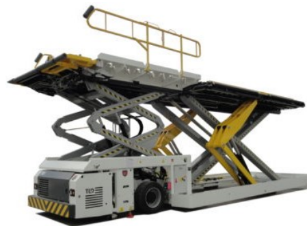
(b) An example of a main deck loader [81].
