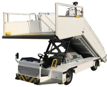
Figure A.12: An example of mobile boarding stairs [81].
