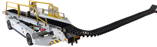
(b) An example of a belt loader equipped with a power stow [57].
