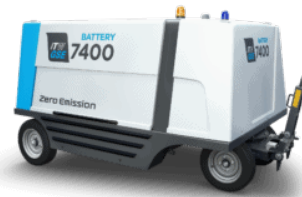
(c) An example of a mobile GPU [81].
