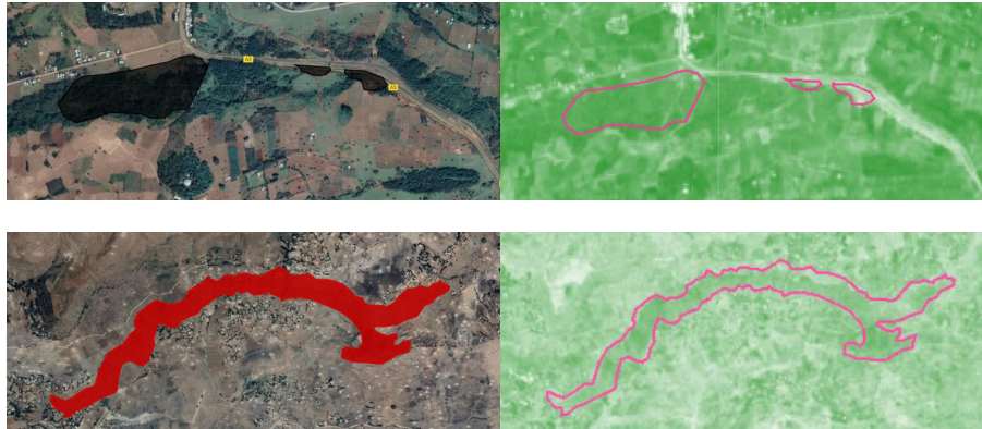
Figure 11. An example of two project sites highlighted in pink and the relatively high resolution Sentinel NDVI image (visible light RGB image on the left)
