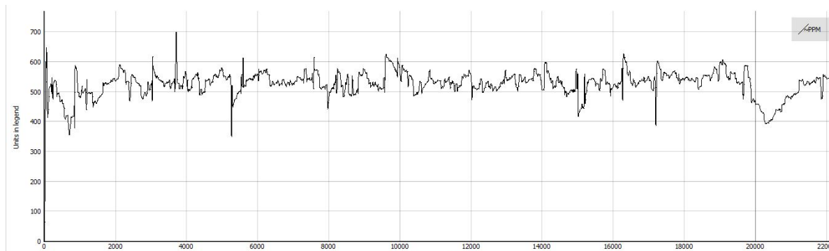
Figure 3.11: CO 2 concentration inside climate chamber during an Airfarm experiment.
