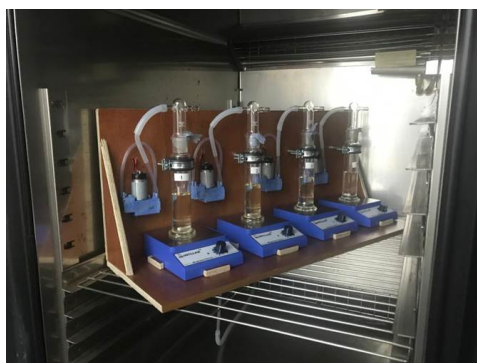
Figure 3.7: final assembly of Airfarm setup inside the climate chamber
