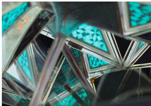
Figure 4 Phototropia in its final assembly showing skin of electroluminescent displays facing down- and dye-solar cells upwards, bioplastic pillars and electroactive polymers populating the ground (Photos: Manuel Kretzer, 2012).
