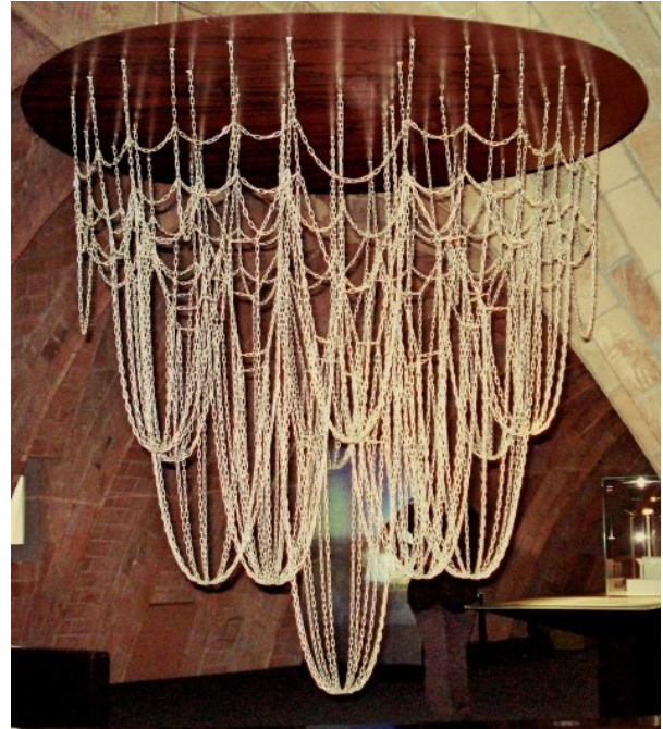
Figure 2.1: Picture of one of Gaudí's hanging chain models, used for the design of compression arches. Source: Little Big Welt, www.littlebigwelt.co.uk/barcelona
