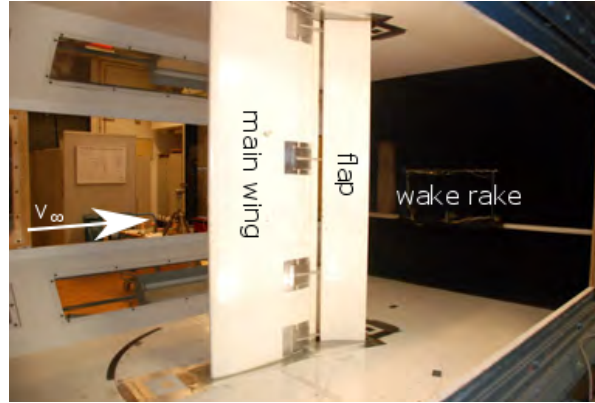
(a) NLF-22 mod-B wing model in the LTT facility at TU Delft (reproduced and annotated from Veldhuis et al. [165])
