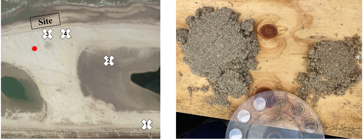
Figure 15: The four sediment sampling locations at the Sand Engine (left panel). A sand ruler used on-site to estimate grain size characteristics (right panel).
