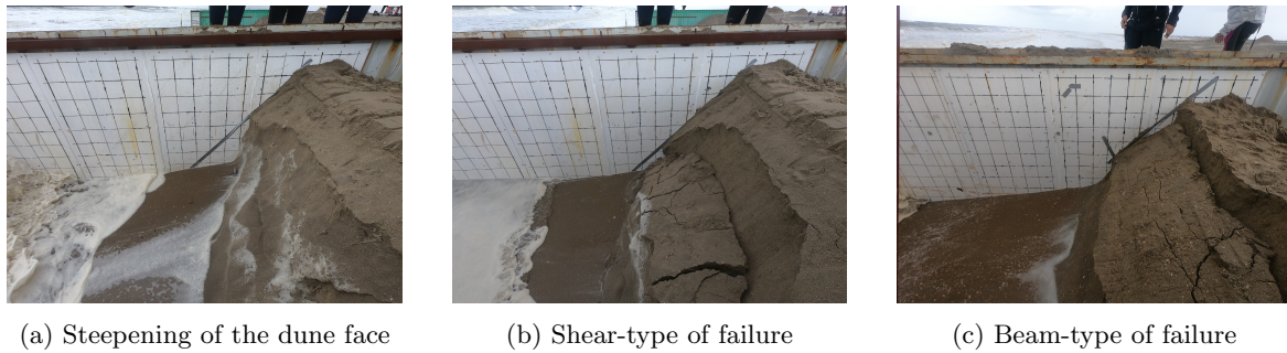
Figure 30: Observations of geotechnical aspects influencing erosion mechanisms for run 3R on Monday 26-09-2022. (a) A very steep profile. (b) Shear-type of failure, when the weight exceeds the shear strength. (c) Beam-type of failure, when a tension crack is developed landwards.
