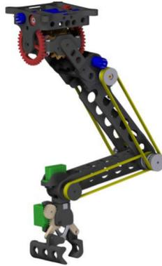
Fig. 2. PULSAR robot arm (motors in blue, servos in green)
