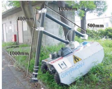
Figure 2.7: Pantograph based manipulator for demining. Source: [16]
