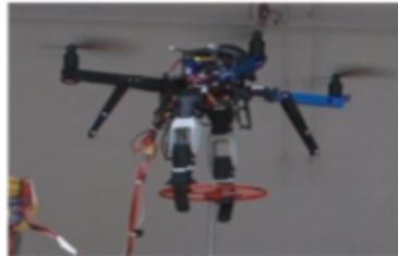
**Figure 2.17:** Dual arm aerial manipulation for valve turning. Source: [8]
