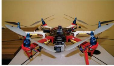
**Figure 2.13:** Hexrotor with tilted propellers for force exertion. Source: [35]
