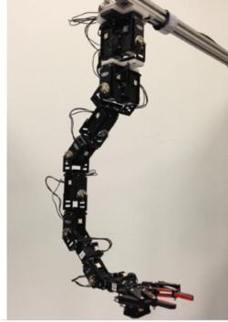
**Figure 2.11:** Hyper-redundant manipulator for UAVs. Source: [7]
