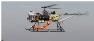
**Figure 2.10:** Redundant manipulator attached to helicopter. Source: [2]
