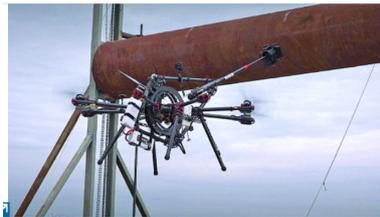
Figure 2.5: Inspection UAV with rotating batteries for force balance. Source: [12]
