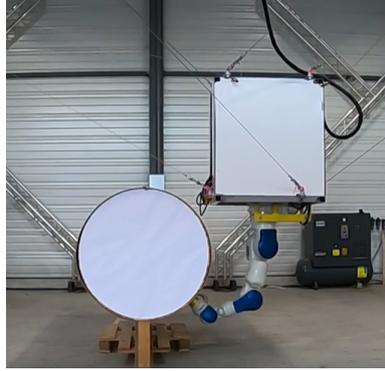
**Figure 2.14:** Cogiro Cable Robot with industrial manipulator. Source: [37]
