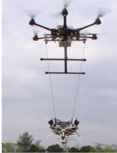
**Figure 2.23:** UAV with fans to suppress swinging. Source: [43]
