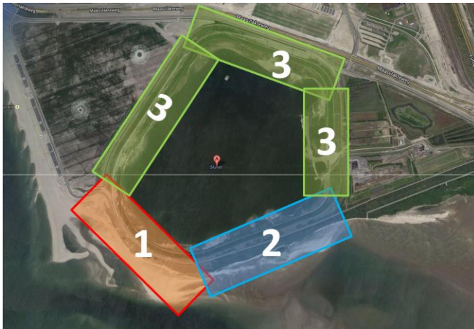
Figure 75 ... Different dam sections (#1 red = North Sea dams, #2 blue = West-Voorne dams, #3 Maasvlakte dams)
