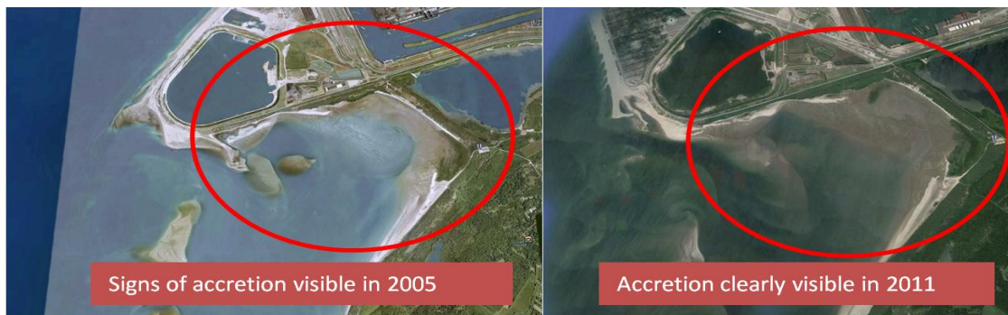
Figure 54 ... Accretion visible in the area east-ward of the Slufter
