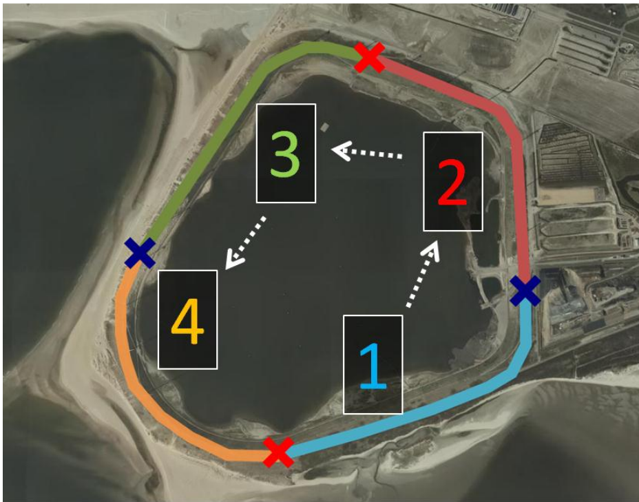
Figure 130 ... Placement of the sheet piles, numbers indicating sections, X marks indicating sheet pile borders (ArcGis, 2013)
