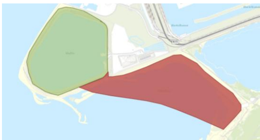
Figure 161 ... Expansion of the Slufter (adjusted from the design of alternative 3, expansion indicated in red)
