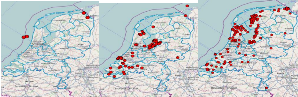
Figure 20 ... Current wind energy projects in the Netherlands from left to right, >50 MW (1st), 10-50 MW (2nd), 1-10 MW (3rd) (Rijkswaterstaat, www.w-i-n-d.nl , 2012)
