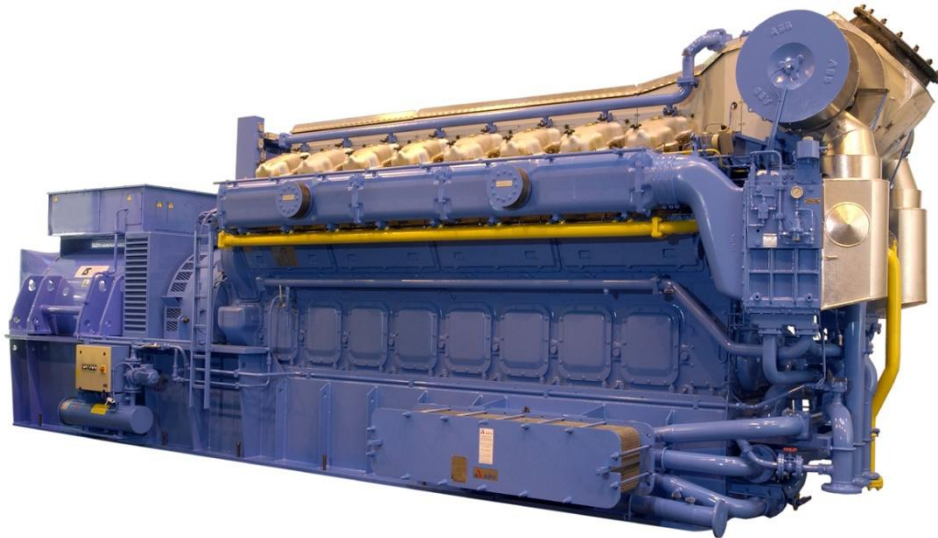
Figure 3: Lean burn gas engine, manufactured by Rolls Royce
