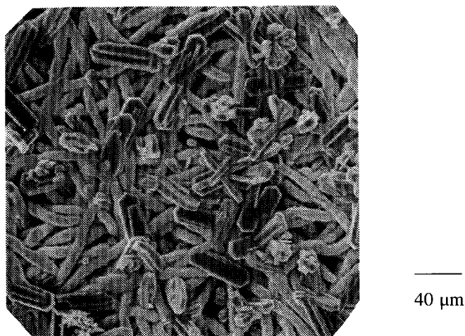
Figure 17 SEM-picture of small MFI crystals on top of a two-layer stainless steel support, prepared according to SS-2
