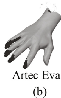
Fig. 20. (a) The scanning process of using an Artec Eva® scanner. (b) The 3D scan captured by the Artec Eva® scanner.
