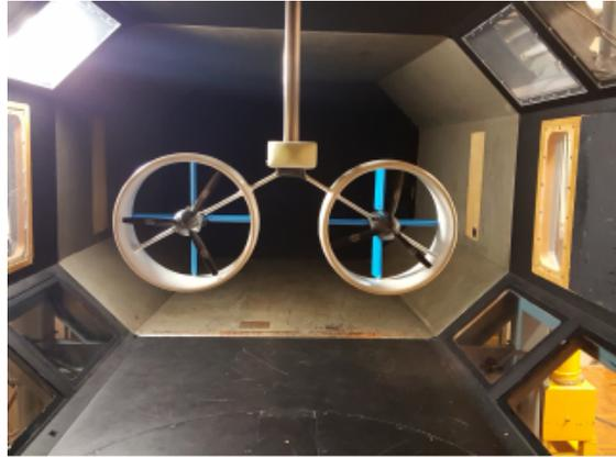
Figure 3.8: Front view of the DUUC model mounted in the test section
