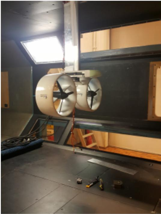
Figure 3.7: Geometric view of the DUUC model mounted in the test section
