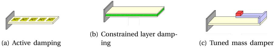
Figure 1.2.: Different damping methods [3]
