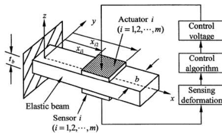
Figure 1.3.: Active vibration control with collocated transducer setup [5]
