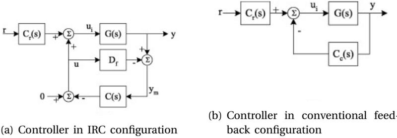
Figure 2.5.: Integral resonant control [5]
