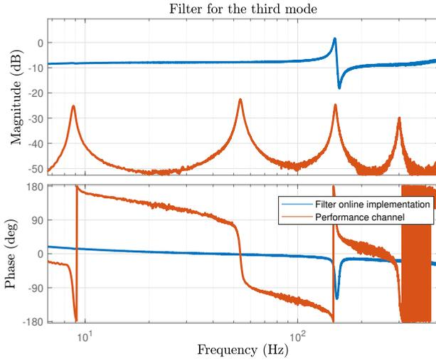
Figure 3.6.: Online implementation of  $T_{u,3}$  and  $T_{y,3}$
