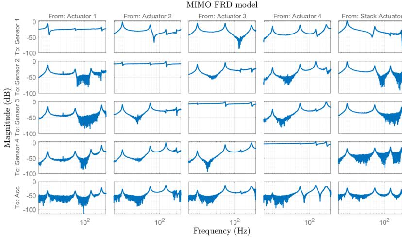
Figure 3.4.: MIMO frequency response function obtained from the experimental setup
