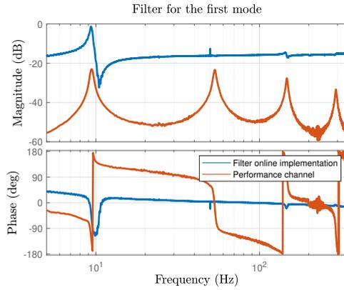
Figure 4.4.: Online implementation of  $T_{u,1}$  and  $T_{y,1}$
