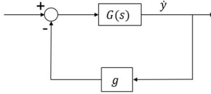
Figure 2.6.: Principle of Direct Velocity Feedback
