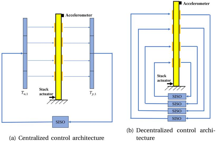
Figure 3.1.: Centralized control and decentralized control architecture
