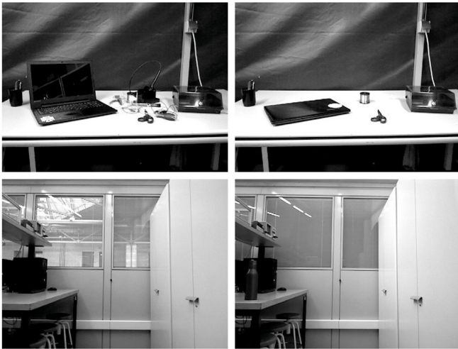
Fig. 1. Examples of changes that can be detected by the proposed algorithm. Handling these changes appropriately allows for more accurate localization.
