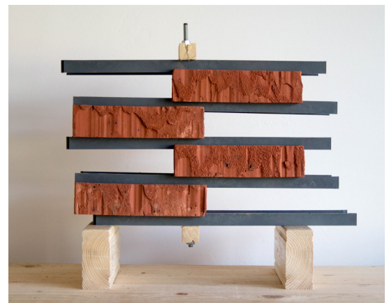
figure 108, Prototype for a quarter bat overlap, using the holes in extruded brick.
