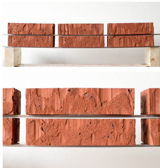
figure 45: Setup for measurements in aluminium. Again the layers don't touch in the middle.
