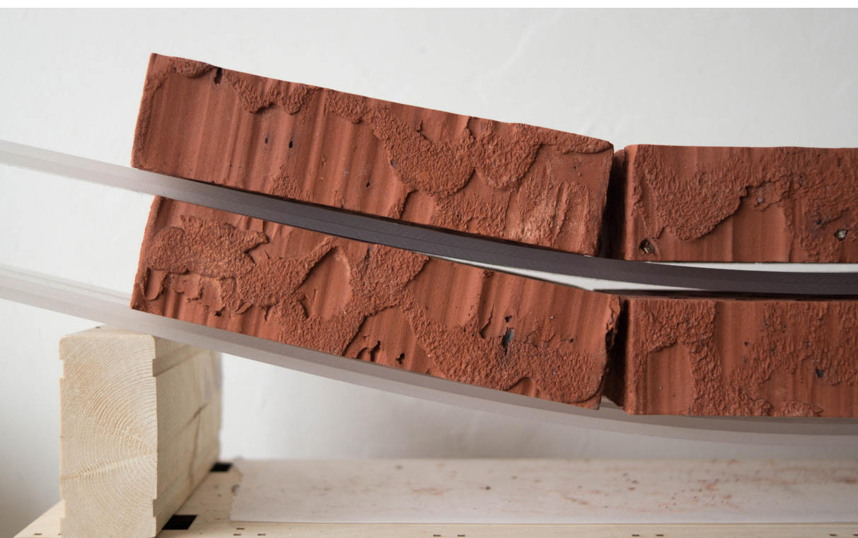
figure 46: Half of a span with two layers.
