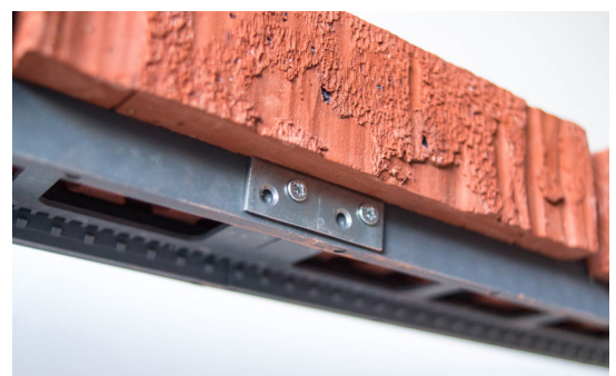
figure 60, Prototype to see the effect of fixed head-joints. Fixating joints with screws is cumbersome, slow and imprecise.
