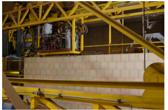
figure 03, Automated wall production at Ploegsteert factory.
