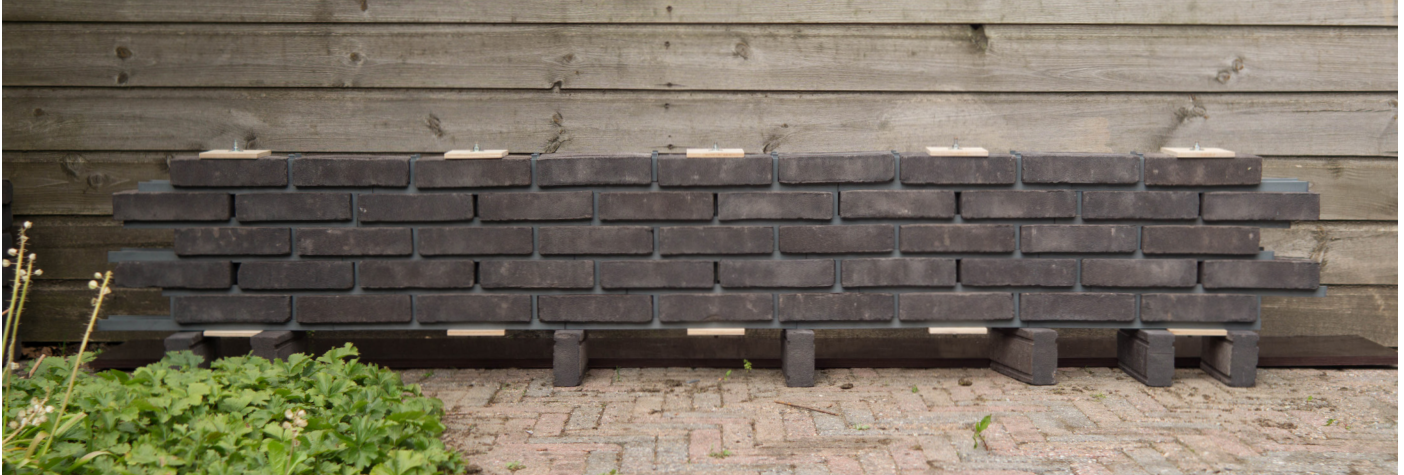
Setup 1: 5 courses, 5 tension rods, only standard profiles
