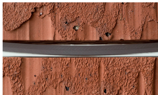
figure 44: The layers don't touch in the middle, with PMMA strips 3 bricks wide.
