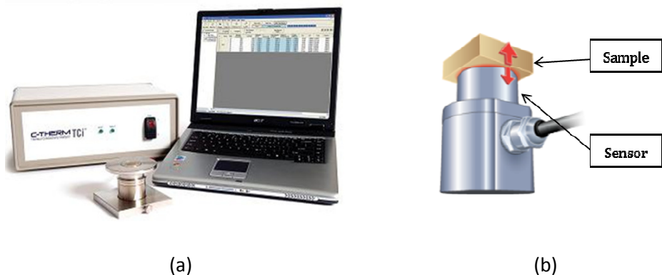
(a) (b) Figure 3.6 (a) Thermal Conductivity Analyzer instrument (C-THERM TCi™); (b) Schematic diagram of TCi set-up.
