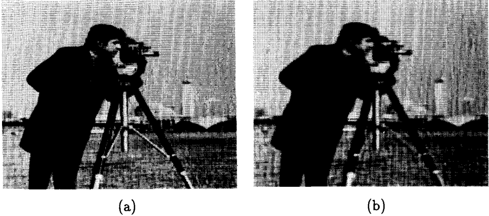
Figure 8.2: Restoration of the motion blurred cameraman image ( L=8 ) using identified parameters: (a) SNR=40 dB; (b) SNR=20 dB.
