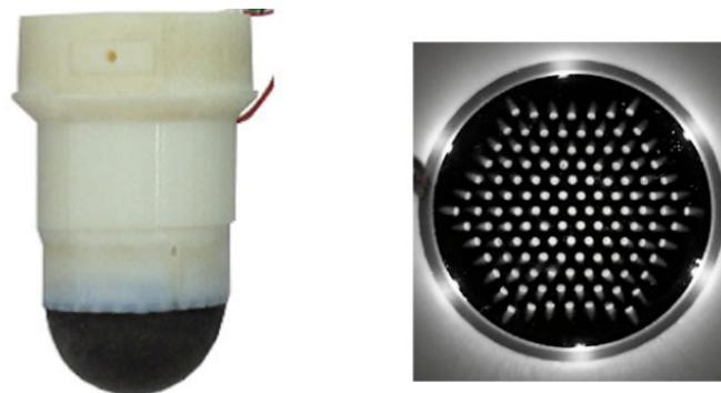
Figure 3.7: Left: The TacTip sensor as shown in [16]. Right: The corresponding output which can be obtained by tapping across various surfaces.
