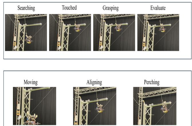
Fig. 8: Illustration of experiment trajectories and states. The top figure depicts state transitions during an experiment incorporating tactile feedback, while the bottom figure showcases the drone attempting an open-loop perch.
