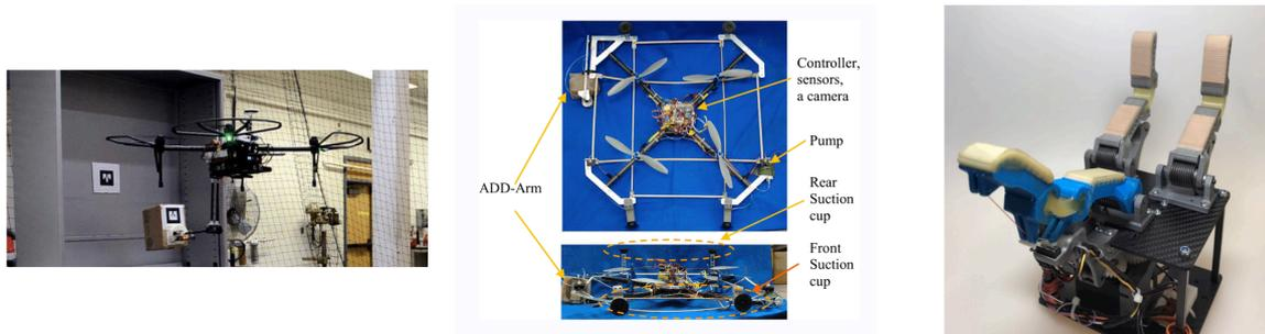
Figure 3.2: From left to right, A drone, developed by Garmella et al [22], utilizing a magnetic effector to pick up a magnetic object, The layout of a drone, developed by Tsukagoshi et al. [11] that utilizes suction cups to be able to attach itself to a door, An ultra-fast closing gripper developed by McLaren et al. [21] that is used for both perching and handling object.
