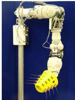
Figure 3.6: The BIOTACT Whisker Tactile sensor developed at Bristol Robotic Laboratory [25].
