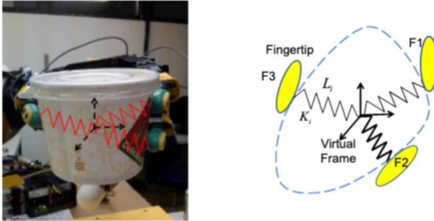
Figure 3.9: Left: The robot used by Li et al. [46] for their experiment with object-level impedance controllers. Right: A schematic showing the distribution of fingertips and the location of the defined *Virtual Frame*
