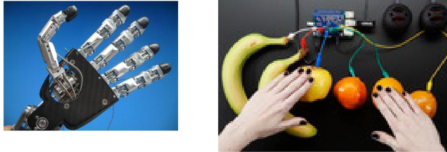
Figure 3.5: Left: The ICub sensor developed by Schmitz et al. [30] attached to a robotic hand. Right: the Adafruit sensor being utilized to detect touch when fruit are being held.
