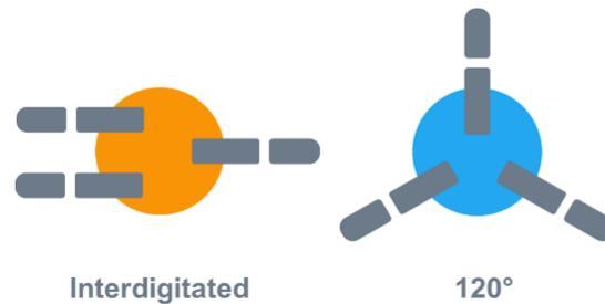
Figure 3.3: Different palm configurations that can be used during the design of the gripper [21]
