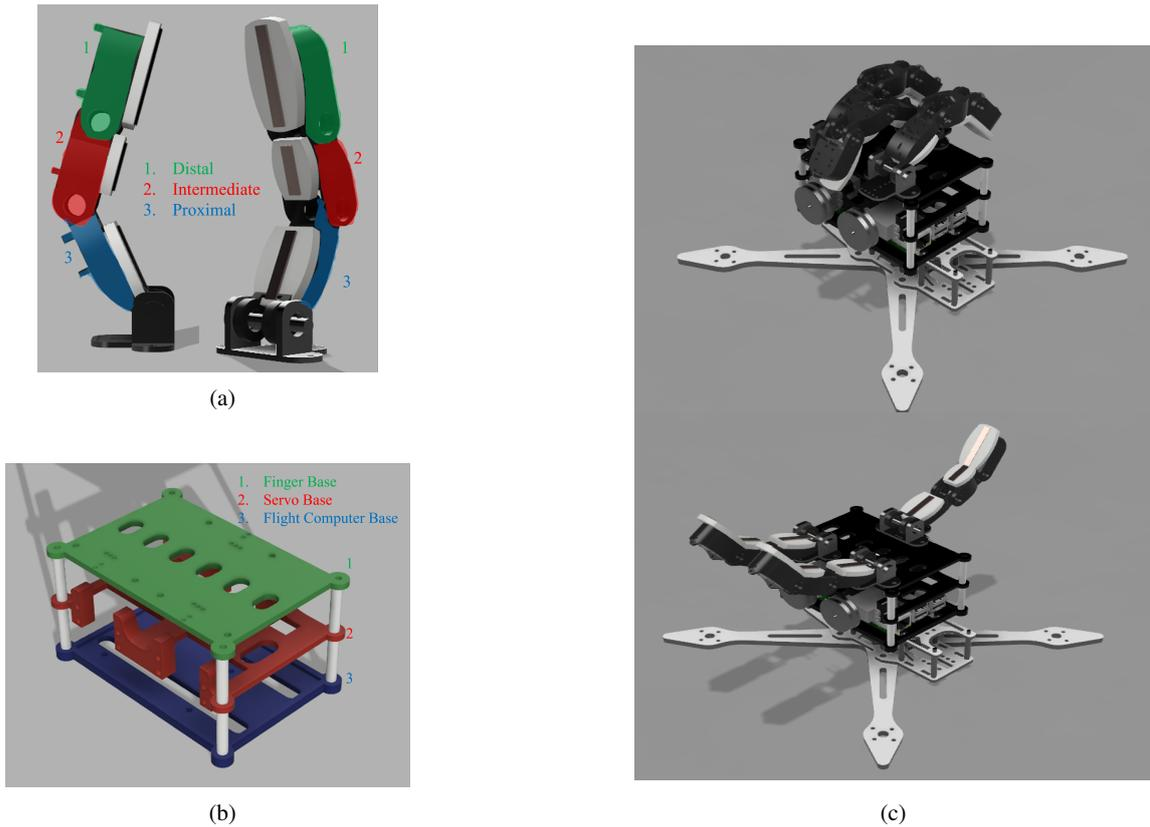
Fig. 2: (a) Renders of the bio-inspired fingers attached to a base, on the left is a side view showing the tendon routing needed to actuate the finger. On the right is a full view of the finger, including the sensing pads. The phalanges are numbered and color coded (b) Rendering of the stack configuration that is mounted atop the drone. Each base is numbered and color coded. (c) Renders of the drone in both closed state (top) and open state (bottom).
