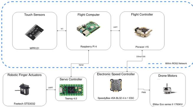
Fig. 4: Onboard drone communication depicted through the flight stack architecture. Defined communication protocols govern interactions between subcomponents, a distinction is made between components within the ROS2 network and outside of it.
