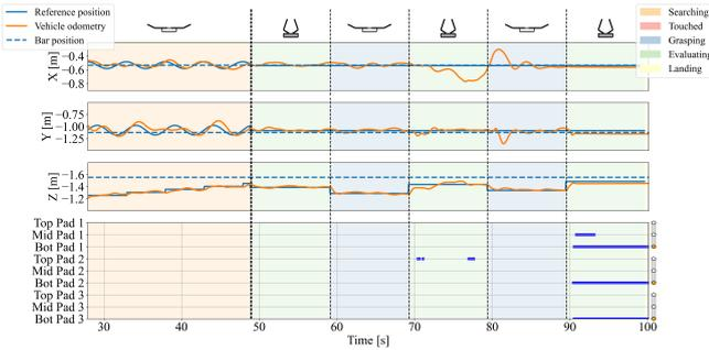
Fig. 13: The drone’s capability to assess a grasp and adapt its goal position is demonstrated. Following each unsuccessful attempt, the grasp evaluator elevates the drone’s altitude, continuing until the evaluator identifies a successful grasp. The concluding segment of the plot displays the final tactile configuration attained by the system.
