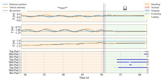
Fig. 11: The behavior of the system throughout a single trial is depicted, showcasing the dynamic changes in its state based on events. The state machine transitions are visualized, providing insights into the system’s response to various cues. Additionally, the state of the tactile sensing pads at the conclusion of the trial is presented at the end of the plot.
