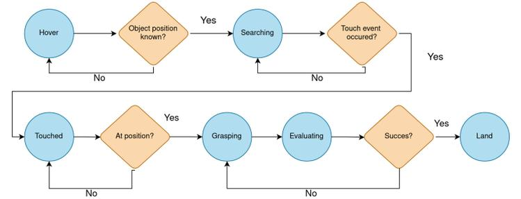
Fig. 6: Flowchart of the state machine
