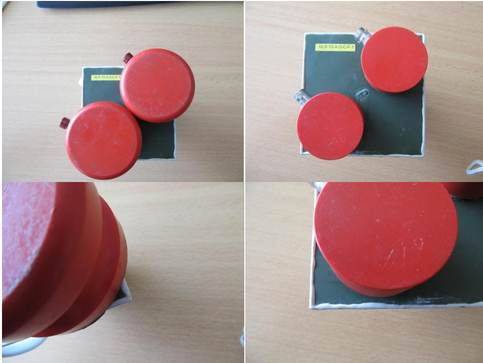
Figure 52. Left: Placement on the laboratory coupon of old handheld sensor design. Right: Placement on the laboratory coupon of new handheld sensor design.
