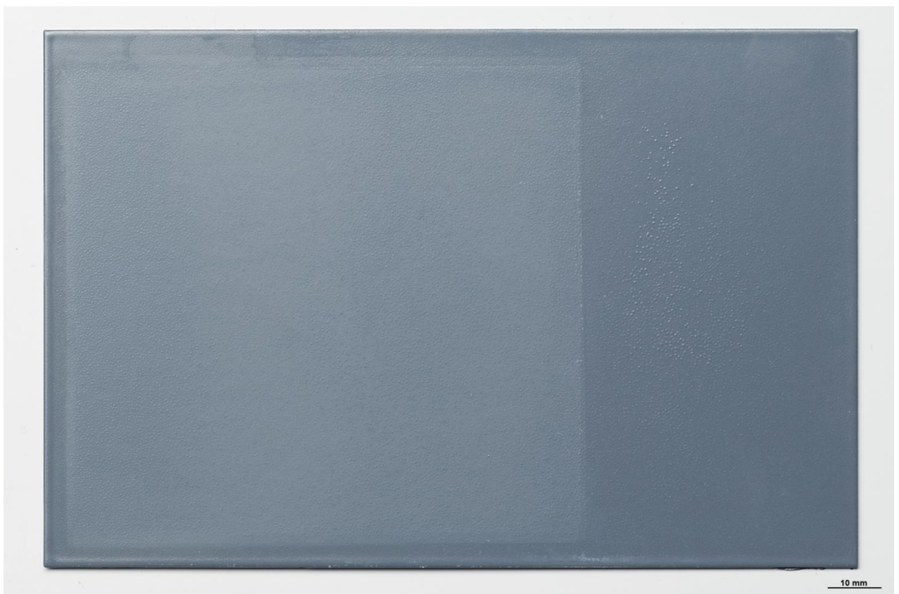
Figure 31. Blister formation on coupon 2-5-4-1 after 110 days of exposure in the UV condensation cabinet.
