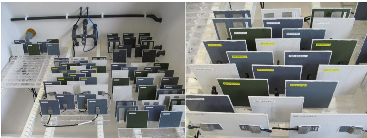
Figure 20. The laboratory coupons placed in the salt-spray cabinet.
