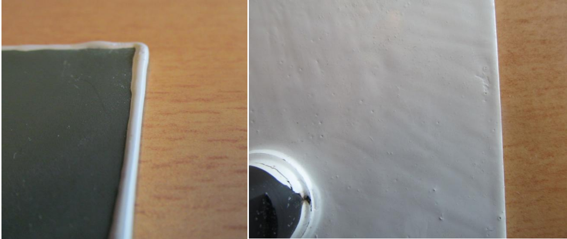
Figure 19. Epoxy coating for the protection of underside and edges of the coupon.
